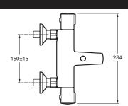
Product Specification: Thermostatic single-lever wall-mount bath/shower mixer. 45714D. Collection: JULY. Installation: Wall-mount. Flow rate: 21 I/min. Connection: With connectors and wall escutcheons. Safety stop at 37°C. maximum temperature 50°C. Non-return valve on supply connections. Connectors with wall escutcheons. Anti-scale aerator. Discreetly-positioned automatic diverter.
