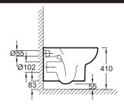
Product Specification: Wall-hung WC pan 54 x 36.5 cm. 4570K. Collection: REACH. Dimensions: 54 x 36.5. Weight: 26 kg. Material: Ceramic. Installation: Wall-hung. Rimless. Projection 54 cm. Low flush 2.6/4 l or 3/6 l possible.
