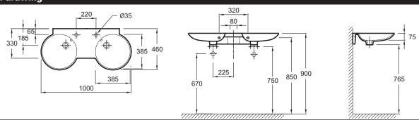
Product Specification: 1-hole double basin vanity top 100 cm. 4148K. Collection: SPHERIK. Dimensions: 100 x 46. Weight: 19.1 kg. Material: Ceramic. Installation: Self-supporting or can be mounted on a specific cabinet. Faucet drilling: 1 faucet hole. Fluidity between curved and straight lines. Generous. functional ledge. Contemporary aesthetics with 2 slightly rounded basins. Without overflow hole 4148K-X5. Chromed overflow cap.
