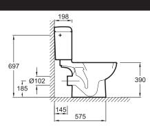
Product Specification: Close coupled WC pan 69.5 x 36 cm. 4101K. Collection: PATIO. Dimensions: 69.5 x 36. Weight: 21.2 kg. Material: Ceramic. Installation: Floor-standing. Lowflush dual at 2.6/4 L or 3/6L. Vario outlet.
