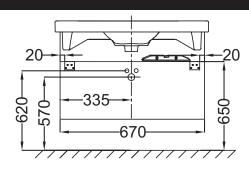
Product Specification: Base unit, 67 cm. 4068K. Collection: REACH. Dimensions: 67 x 48.5 x 53 cm. Weight: 30 kg. Material: Solid color decor or wood decor. Installation: Wall-hung. 2 superimposed lef-hand slow-close drawers. 1 organizer inside upper drawers.
