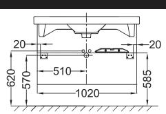
Product Specification: Base unit 102 cm. 4023W. Collection: REACH. Dimensions: 102 x 48.5 x 45. Weight: 29.6 kg. Material: Solid color decor or wood decor. Installation: Wall-hung. 1 slow close drawer. Includes storage basket (L  $28 \times D 37 \times H 17 \text{ cm}$ ) EB197 and divider (L  $55 \times D 32.5 \times H 6.5 \text{ cm}$ ) EB122.
