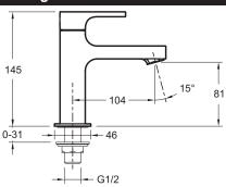
Product Specification: Pillar tap for handwash basin. 37333D. Collection: STRAYT. Installation: 1 hole. Flow rate: 5 l/mn. No drain. Cold water only. Anti-scale aerator. Ceramix disc valves.
