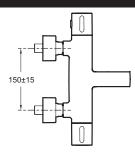
Product Specification: Thermostatic single-lever wall-mount bath/shower mixer. 37037D. Collection: CÜFF. Weight: 3.6 kg. Installation: Wall-mount. Normes: ACS (Certificate of Sanitary Compliance): 10 ACC LY 102. Connection: With connectors and wall escutcheons. Mechanism: Expandable wax cartridge. Hole configuration: 150 ± 15 mm. On temperature handle: Safety stop at 38°. Maximum temperature limited to 50°. Twist-free supply hoses. Integral anti-scale aerator. 5-year guarantee.
