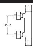
Product Specification: Thermostatic single-lever wall-mount shower mixer. 37035D. Collection: CÜFF. Weight: 3.1 kg. Installation: Wall-mount. Normes: ACS (Certificate of Sanitary Compliance): 10 ACC LY 102. Connection: With connectors and wall escutcheons. Mechanism: Expandable wax cartridge. Hole configuration: 150 ± 15 mm. On temperature handle: Safety stop at 38°. Maximum temperature limited to 50°. Integral anti-scale aerator. 5-year guarantee.
