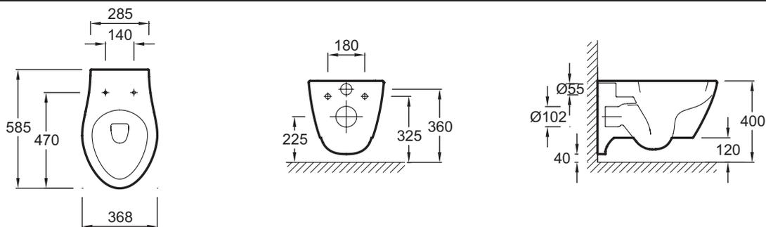
Product Specification: Wall-hung WC pan 58.5 x 37 cm. 3594W. Collection: VIA. Dimensions: 58.5 x 37. Weight: 29.5 kg. Material: Ceramic. Installation: Wall-hung. Toilet with soft, rounded forms. Slow-close ergonomic seat E70012 included. Water saving dual flush 3/6 L.
