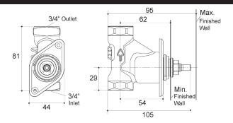
Product Specification: Volume control valve 3/4". 2977-K. Collection: PURISTIC. Flow rate: 106 l/min.
