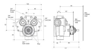
Product Specification: Wall-mount-thermostatic valve 3/4". 2975-KS. Collection: PURISTIC. Flow rate: 65 l/min.
