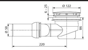
Product Specification: Drain for shower tray Ø 9 cm. 19200. Collection: NO COLLECTION. Weight: 0.6 kg. Flow rate: 42 l/min.
