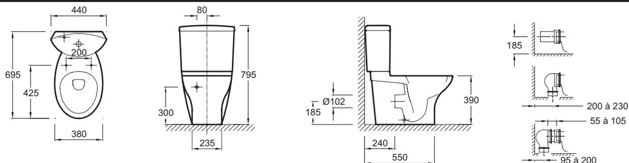
Product Specification: WC pan 69.5 x 38 cm. 19077. Collection: PRESQU'ÎLE. Dimensions: 69.5 x 38. Weight: 35 kg. Material: Ceramic. Installation: Floor-standing. Fixings: Concealed floor fixings included. Soft, classic lines. Slow-close thermostet seat E70003 with metal hinges included. Vario outlet: for any kind of installation (P-trap, S-trap, side outlet).
