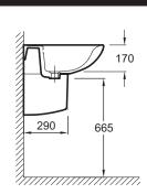
Product Specification: 1-hole washbasin 66 cm. 18909D. Collection: PATIO. Dimensions: 66 x 53. Weight: 17.5 kg. Material: Ceramic. Installation: Self-supporting. Faucet drilling: 1 faucet hole. Functional design with flat and wide ledges.
