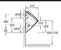
Product Specification: Urinal 53 x 30.6 cm. 18843D. Collection: PRESQU'ÎLE. Dimensions: 30 x 50 x 29. Weight: 13.3 kg. Material: Ceramic. Installation: Wall-mount. Smooth sided. back-to-wall. concealed fixings (included), for easier cleaning. Siphon action, no rising odours, Concealed supply and drainage, Cover and metal hinges included, for elegant look.
