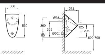
Product Specification: Urinal. 18842D. Collection: REACH. Dimensions: 30.5 x 53 x 31. Weight: 13.3 kg. Material: Ceramic. Installation: Wall-mount. Smooth sided. back-to-wall. concealed fixings (included). for easier cleaning. Siphon action. no rising odours. Concealed supply and drainage.
