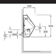
Product Specification: Urinal 30 x 62 x 32 cm. 18645W. Collection: PATIO. Dimensions: 30 x 62 x 32. Weight: 18 kg. Material: Ceramic. Installation: Wall-mount. Fully concealed equipment for added aesthetic and hygiene. Built-in inlet. Built-in drainage. Delivered with full equipment. Fixing brachets. water spreader. hose. strainer waste. P trap siphon.
