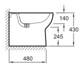
Product Specification: Bidet 57 x 36.5 cm. 18569W. Collection: REACH. Dimensions: 57 x 36.5. Weight: 24.1 kg. Material: Ceramic. Installation: Floor-standing. Faucet drilling: 1 faucet hole. Smooth-sided. back-to-wall. no dirt traps for perfect hygiene. Contemporary design. Chromed overflow cap.
