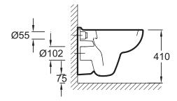
Product Specification: Compact wall-hung WC pan 48.5 x 36.5 cm. 18560W. Collection: REACH. Dimensions: 48.5 x 36.5. Weight: 17.6 kg. Material: Ceramic. Installation: Wall-hung. Installation solution for small spaces. Smooth siphon for perfect upkeep. Ergonomic seat and metal hinges E70009 or optional slow-close seat E70011. Contemporary design. Closed glaze rim.
