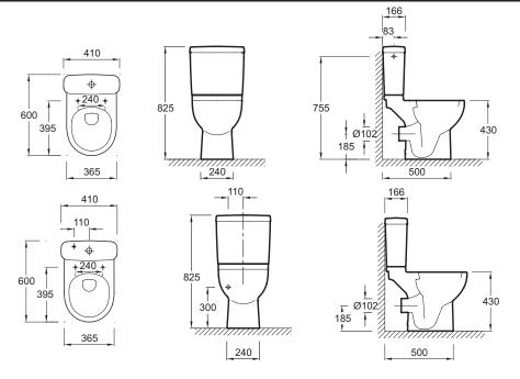
Product Specification: Compact WC pan 60 x 36.5 cm. 18557K. Collection: REACH. Dimensions: 60 x 36.5. Weight: 27.9 kg. Material: Ceramic. Installation: Floor-standing. Comfort height 43 cm. 3/6L flush.
