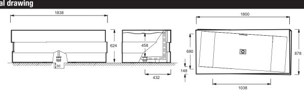
Product Specification: Lithocast bath, freestanding, 185 x 90 cm. 1801K. Collection: ASKEW. Dimensions: 185 x 90. Weight: 260 kg. Material: Lithocast. Installation: Freestanding. Volume: 379. Shape: Rectangular. Integrated overflow. Incl. clicker waste.
