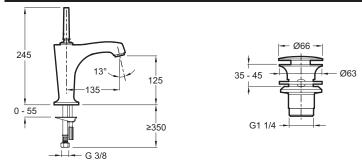
Product Specification: Single-lever washbasin mixer. 16230D-4. Collection: MARGAUX. Weight: 2.7 kg. Installation: 1 hole. Flow rate: 8 l/min. Connection: With supply hoses. Mechanism: Ceramic Joystick disc cartridge. Margaux offers a unique blend of traditional design elements and modern fluidity to complement eclectic design interiors with refreshed sophistication. Joystick lever. Anti-scale aerator. No lift rod.
