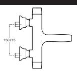
Product Specification: Thermostatic single-lever wall-mount bath/shower mixer. 16215D-9. Collection: MARGAUX. Weight: 4.8 kg. Installation: Wall-mount. Flow rate: 19 l/min. Connection: With connectors and wall escutcheons. Hole configuration: 150 ± 15 mm. Margaux offers a unique blend of traditional design elements and modern fluidity to complement eclectic design interiors with refreshed sophistication.
