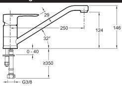
Product Specification: Single-lever sink mixer. 16084D-4. Collection: JULY. Weight: 1.2 kg. Installation: 1 hole. Flow rate: 12 l/min. Mechanism: Ceramic disc cartridge with temperature and flow limiter. Spout 250 mm. Temperature limiter ring. Anti-scale aerator.
