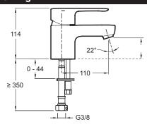
Product Specification: Single-lever washbasin mixer, no drain. 16027D-4ND. Collection: JULY. Weight: 1.2 kg. Installation: 1 hole. Flow rate: 12 I/min. Flow rate: 12 I/min. Mechanism: Ceramic disc cartridge with temperature and flow limiter. The July range combines compact curved lines with robust manufacturing for hassle-free installation and use. Sensitive flow control. Temperature limiter ring. Anti-scale aerator. Smooth body. no lift rod. no waste.
