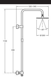
Product Specification: Shower column with round showerhead. 15370D. Collection: TOOBI. Weight: 7 kg. Installation: Wall-mount. Round showerhead Ø 20 cm. Shift Ellipse handshower. Toobi single control mixer. Discretly positioned diverter. Smooth. anti-twist metal look hose. Cold body scald protection. Flow rate: showerhead 10 l/min. handshower 9 l/min.
