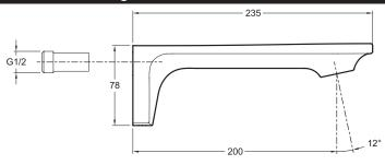
Product Specification: Wall-mount bath filler. 14795D. Collection: STANCE. Installation: Wall-mount. Flow rate: 30 I/min. Anti-scale aerator.
