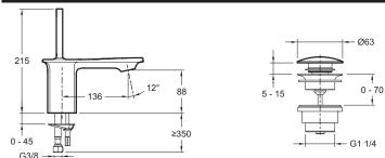
Product Specification: Single-lever washbasin mixer. 14760D. Collection: STANCE. Weight: 3.4 kg. Installation: 1 hole. Flow rate: 5.7 l/min. Connection: With supply hoses. Pure design. straight lines. Joystick lever. No lift rod.
