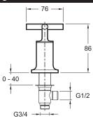
Product Specification: Handle kit for bath mixer. 14429D-3. Collection: PURISTIC. Installation: Wall-mount. Flow rate: 43 I/min. Cross handles. Incl. Wall-mount mixing valve. Ceramic disc valves.
