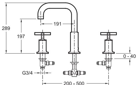
Product Specification: 3-hole deck-mount bath mixer. 14428D-3. Collection: PURISTIC. Weight: 4 kg. Installation: 3 holes. Flow rate: 30 l/mn. Mechanism: Ceramic disc heads. Puristic brassware combines the strength of simple, architectural forms with sensual lines and careful detailing. Elements of relaxed minimalism are honest interpretations of classic modernity.
