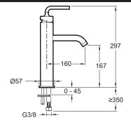
Product Specification: Tall single-lever washbasin mixer. 14404D-4A. Collection: PURISTIC. Weight: 3.4 kg. Installation: 1 hole. Flow rate: 7.5 l/min. Connection: With supply hoses. Mechanism: Ceramic disc cartridge. Puristic brassware combines the strength of simple. architectural forms with sensual lines and careful detailing. Elements of relaxed minimalism are honest interpretations of classic modernity. Temperature limiter ring. Anti-scale aerator.
