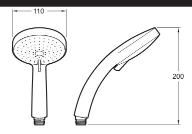
Product Specification: 5-spray handshower Ø 110 mm. 12914D. Collection: CITRUS. Weight: 0.7 kg. Flow rate: 9.5 I/min. Anti-scale system. Flow control.
