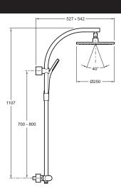
Product Specification: Thermostatic shower column. 11717D. Collection: OBLO. Weight: 12.1 kg. Installation: Wall-mount. E0 small handshower (flow rate: 10 L/min). FLOW RATE: shower head 10l/min, handshower 10 l/min.
