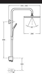
Product Specification: Shower column with square showerhead. 11716D. Collection: EO. Weight: 6.2 kg. Installation: Wall-mount. Flow rate: 11 I/min. Shower column with square showerhead. ABS showerhead: 280 x 280 mm (flow: 11 L/min). Descretly positionned diverter. Anti-scale EO Small handshower (flow rate: 10 L/min). 2 smooth metal look hoses.
