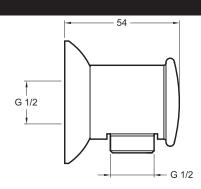
Product Specification: Square shower elbow. 11627D. Collection: NO COLLECTION. Weight: 0.5 kg. Installation: Wall-mount. Brass construction.
