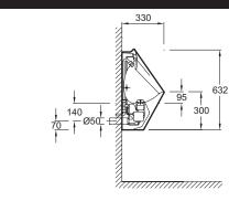
Product Specification: Urinal with sensor. 1088K. Collection: PATIO. Dimensions: 30 x 62 x 32. Weight: 20.7 kg. Material: Ceramic. Installation: Wall-mount. Electronic control for hygiene and water saving.
