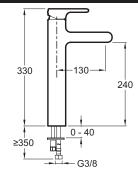
Product Specification: Tall single-lever monobloc basin mixer. 10861D. Collection: SINGULIER. Weight: 3 kg. Installation: 1 hole. Flow rate: 7 l/min. Connection: With supply hoses. Mechanism: Ceramic disc cartridge. The Singulier range combine elegant. sensuous lines with graceful curves that come together delicately to create a serene. understated look and tranquil sensibility.. Temperature limiter ring. Sensitive flow control. Anti-scale aerator. No lift rod.
