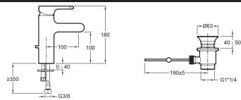
Product Specification: Single-lever monobloc basin mixer. 10860D. Collection: SINGULIER. Weight: 2.7 kg. Installation: 1 hole. Flow rate: 13 l/min. Connection: With supply hoses. Mechanism: Ceramic disc cartridge. The Singulier range combine elegant. sensuous lines with graceful curves that come together delicately to create a serene. understated look and tranquil sensibility.. Temperature limiter ring. Sensitive flow control. Anti-scale aerator. Side lift rod.
