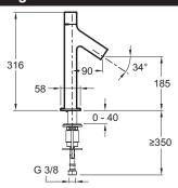
Product Specification: Tall single-lever basin mixer. 10379D. Collection: OBLO. Weight: 2.9 kg. Installation: 1 hole. Flow rate: 8 l/min. Connection: With supply hoses. Mechanism: Sequential cartridge. The simple. ergonomic design offers a sleek. modern appeal with a European influence. Integrated anti-scale aerator. With sequential cartridge.
