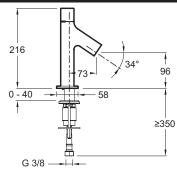
Product Specification: Single-lever basin mixer. 10378D. Collection: OBLO. Weight: 2.1 kg. Installation: 1 hole. Flow rate: 8 l/min. Connection: With supply hoses. Mechanism: Sequential cartridge. The simple. ergonomic design offers a sleek. modern appeal with a European influence. Integrated anti-scale aerator. With sequential cartridge.
