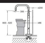
Product Specification: Bath mixer. 10129-4. Collection: PURISTIC. Installation: Floor-mount. Flow rate: 23 l/min. handshower 9 l/min. Puristic brassware combines the strength of simple. architectural forms with sensual lines and careful detailing. Elements of relaxed minimalism are honest interpretations of classic modernity. With sequential cartridge.
