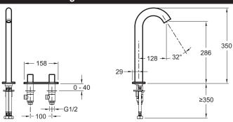
Product Specification: Tall 2-handle 3-hole basin mixer. 10094D. Collection: OBLO. Weight: 3.2 kg. Installation: 3 holes. Flow rate: 6 l/min. Mechanism: Ceramic disc heads. The simple. ergonomic design offers a sleek. modern appeal with a European influence. Integrated anti-scale aerator. Fixed spout separated from handles on plate. Rectangle plate: 158 mm x 58 mm.
