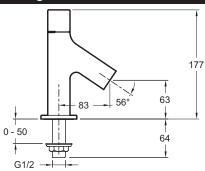
Product Specification: 1-hole handwash basin mixer. 10092D. Collection: OBLO. Weight: 0.8 kg. Installation: 1 hole. Flow rate: 6 l/min. Mechanism: Ceramic disc heads. The simple. ergonomic design offers a sleek. modern appeal with a European influence. Integrated anti-scale aerator.
