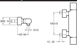
Product Specification: Thermostatic single-lever shower mixer. 10091D. Collection: OBLO. Weight: 3.1 kg. Installation: Wall-mount. Flow rate: 13 I/min. Connection: With connectors and wall escutcheons. Mechanism: Thermostatic cartridge with dilatable wax. Hole configuration: 150 ± 15 mm. The simple. ergonomic design offers a sleek. modern appeal with a European influence. Safety stop at 38° C. temperature limited to 50° C.. Metal handles with laser marking.
