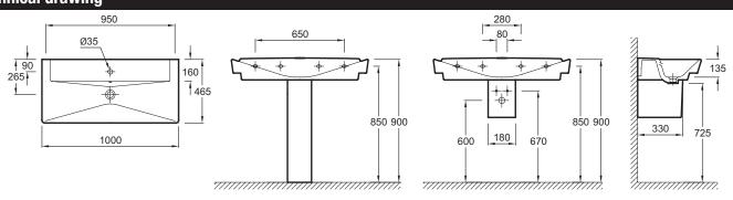
Product Specification: 1-hole vanity top 100 cm. 5026K. Collection: RÊVE. Dimensions: 100 x 46.5. Weight: 34.3 kg. Material: Ceramic. Installation: Self-supporting. Can be mounted onto specific cabinet. with or without pedestal/shroud. Faucet drilling: 1 central faucet hole. Wide ledge for optimal comfort of use. Combination of straight lines and softened angles. Perfect fit with cabinet. Without overflow 5086K. With 3 tap holes 5026K-8. Chromed overflow cap.
