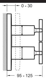
Product Specification: Classic trim for built-in bath/shower mixer. 98732D. Collection: MODULO. Installation: Built-in. Flow rate: 26 I/min. Incl. thermostatic and flow-control valve. Instantaneous water heater suitable. Filter and non-return valves. DVGW NW-6512CP0430.
