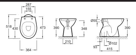
Product Specification: Ducted pan S-trap. 15552K. Collection: BRIVE. Dimensions: 51 x 36. Installation: Independent. S-trap outlet. 2-volume flow technique 3/6 l.
