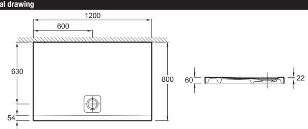
Product Specification: Extra-slim rectangular ceramic shower tray 120 x 80 x 6 cm. N114K. Collection: REACH. Dimensions: 120 x 80 x 6. Weight: 44.5 kg. Material: Ceramic. Installation: Floor-standing or inset. Floorstanding or inset. Anti-slip glaze. Order with special drain and cover 9276K. Waste Ø 90 mm.
