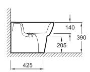
Product Specification: Floor-standing bidet. 19963W. Collection: OVE. Dimensions: 55 x 36. Material: Ceramic. Installation: Floor-standing. Faucet drilling: 1 faucet hole. Fixings: Concealed floor fixings included. Design with soft. classic curves. Smooth-sided. back-to-wall with concealed side fixings. for perfect hygiene and aesthetics. Chromed overflow cap.
